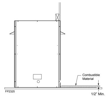
Figure 7 -Floor Clearance above Combustible Flooring Material
