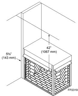
Figure 3 - Sidewall and Ceiling Clearances
