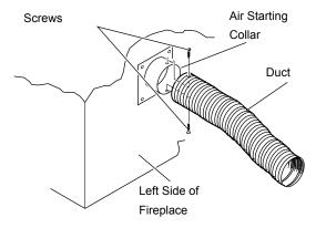
Figure 27 - Attaching Outside Duct to Starting Collar
