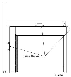
Figure 15 - Location of Nailing Flanges and Floor Screws
