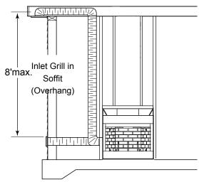
Figure 23 -Concrete Slab Installation (Optional Outside Air Runs)
