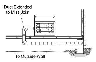
Figure 24 - Installation Above Basement or Crawl Space
