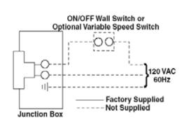
Figure 20a - Wiring Diagram for Junction Box
