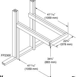
Figure 11 - Framing Specifications for Peninsula Units (Model LPF36)
