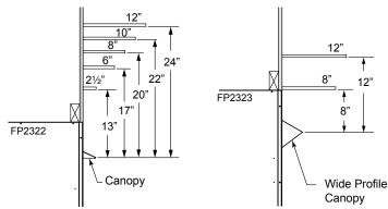
Figure 6 -Minimum Mantel Clearances for Canopy and Wide Profile Canopy
