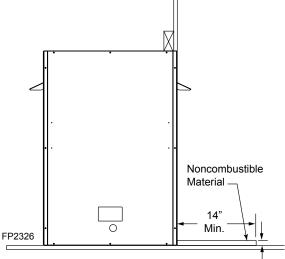
Figure 8 -Floor Clearance above Noncombustible Flooring Material
