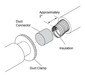
Figure 29 - Install Duct Connector 403
