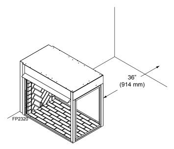
Figure 4 Parallel Wall Clearance
