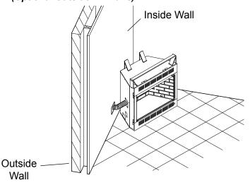
Figure 25 - 45° Corner Installation on Slab Floor
