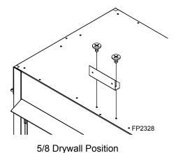
Figure 16 -Nailing Flanges with Different Drywall Depths
