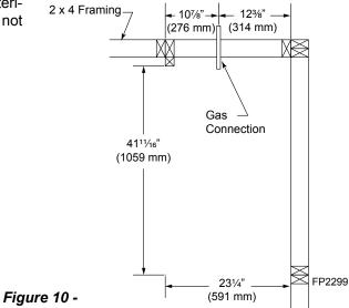
Top View of Framing Specifications for Corner Units (Model LRCF36/LLCF36)
