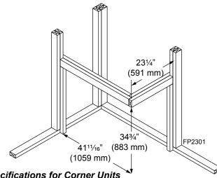
Figure 12 Framing Specifications for Corner Units
