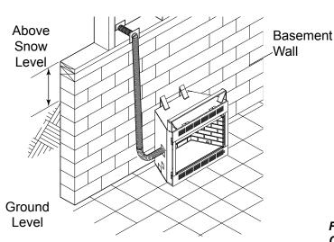
Figure 22 -Basement Installation
