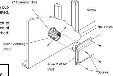
Figure 28 - Combustion Air Assembly for Model No. AK-4
