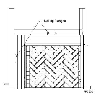
Figure 18 -Location of Nailing Flanges and Floor Screws
