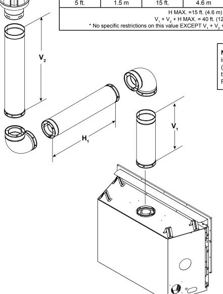
**Note**: There <u>MUST</u> be a 25% reduction in total H when using SLP-FLEX Series (6-5/8 inch) vent except when using the simple up and out installation. See Figure 4.8.
