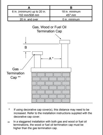
Figure 4.2 Staggered Termination Caps
