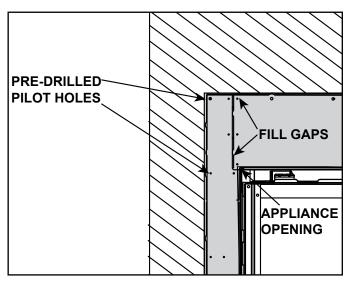
Figure 10.1 Install Non-Combustible Board
