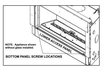
Figure 8.1 Remove Lower Access Panel
