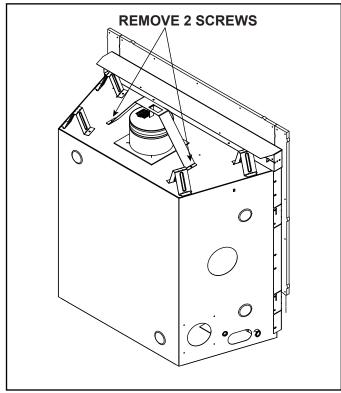
Figure 6.3 JADE32IN - Shipping Support in Shipping Position
