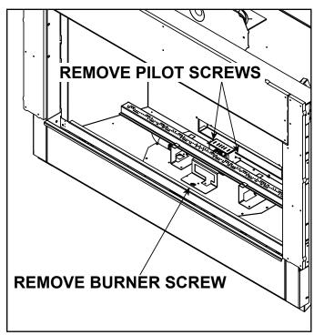
Figure 9.2 Burner Removal
