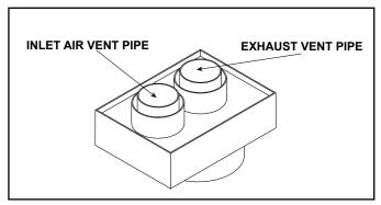
Figure 4.19 Coaxial/Colinear Appliance Adapter (DV-46DVA-GCL)
