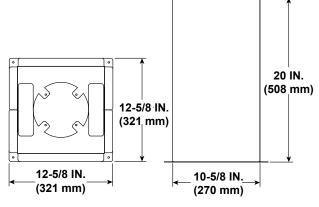
SLP-RDS ROOF DECK INSULATION SHIELD
