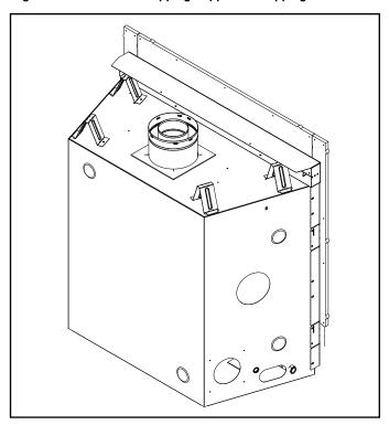
Figure 6.4 JADE32IN - Shipping Support and Seal Cap Removed
