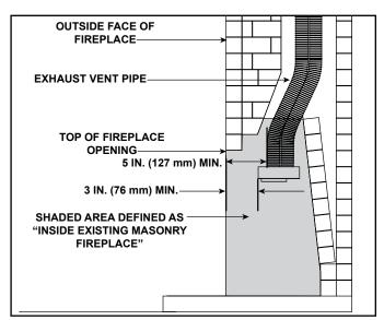
Figure 4.20 Existing Fireplace DV-46DVA-GCL Clearance Requirements
