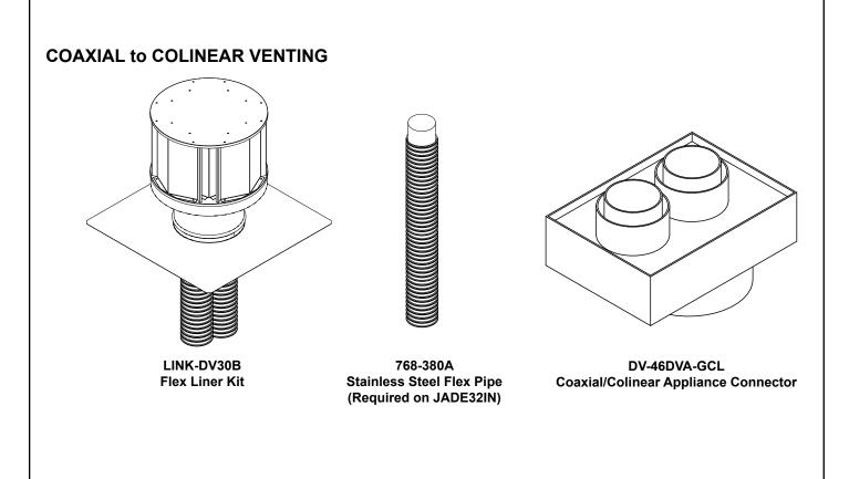
Figure 12.5 Coaxial to Colinear Vent Components
