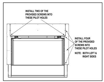
Figure 6.7 Installation of the Side Non-Combustible Components
