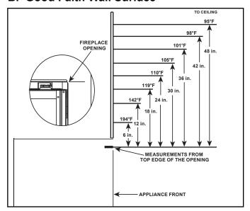
Figure 2.1 Good Faith Wall Surface Temperatures Above Appliance
