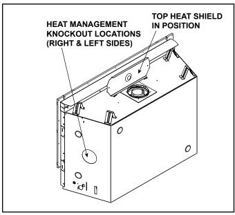
Figure 6.2 JADE42IN/JADE42IL - Top Heat Shield in Position
