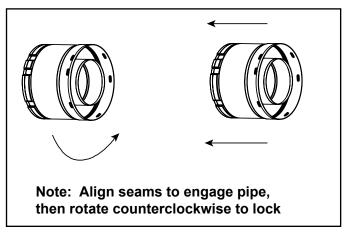
Figure 7.2 Adding Venting Components
