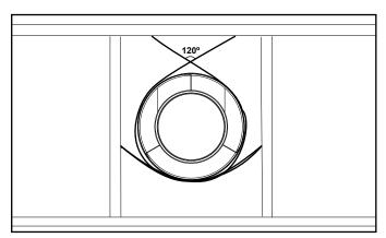
Figure 7.6 Securing Horizontal Pipe Sections
