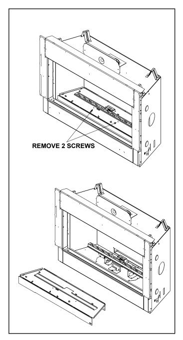
Figure 9.1 Base Pan Removal - JADE42 Shown
