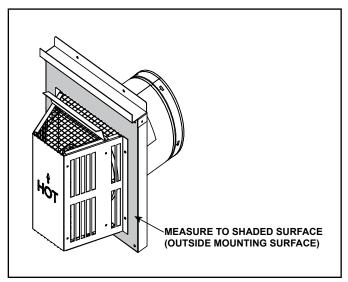
Figure 4.6 Measure to Outside Mounting Surface
