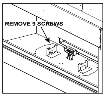
Figure 9.3 Remove Valve Plate
