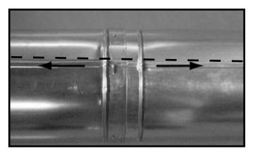
Figure 7.8 Align and Disassemble Vent Sections
