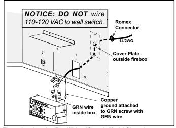
Figure 8.4 Junction Box Wiring (Generic Model Shown)
