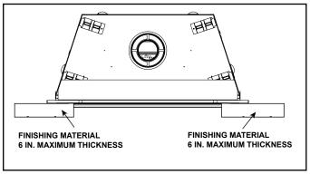
Figure 10.9 Maximum Finish Material Thickness - CFT Decorative Front
