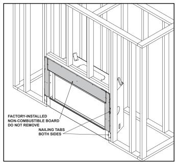
Figure 6.5 Proper Positioning, Leveling And Securing Of Appliance
