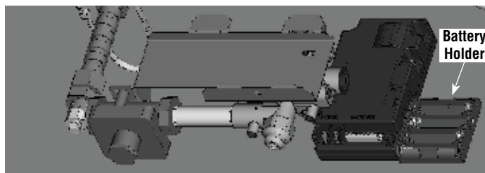
Battery Holder (in control compartment)
